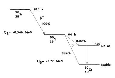
when this happens we will have a 1750-keV photon. This is quite high energy and will often be off scale (not seen) with gamma-detection systems. However, a NaI detector system could easily be adjusted to detect this gamma.
