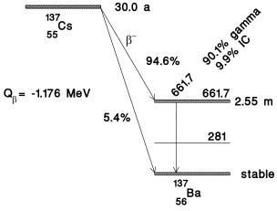
The 661.7-keV level is shown as a bold line and has 2.55 minutes written beside it. This gamma is not prompt. The excited level has a rather significant half-life. This is because the angular momentums of the 661.7 level and the ground state are so different that gamma decay is not easy between the two levels. It is so difficult that it sometimes doesn't even happen; instead, the 661.7-keV of excess energy can be given to
