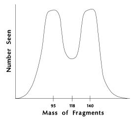
produces a double-humped graph. This indicates a higher likelihood of nonsymmetrical division as compared to symmetrical division (which would produce a single hump). The graph on the right is the approximate graph for  $^{235}$ U.
