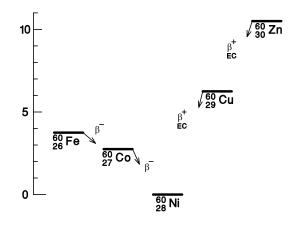
favorable than Z=28, N=32. It is not surprising that Z=26, N=34 is even more energetic. <sup>28</sup>Fe can change a neutron into a proton, electron, and antineutrino. After ejecting the electron and antineutrino it becomes <sup>27</sup>Co. Likewise, <sup>27</sup>Co can convert a neutron to a proton, electron, and antineutrino, eject the electron and antineutrino, and become stable <sup>60</sup>Ni. This is beta-minus decay.
